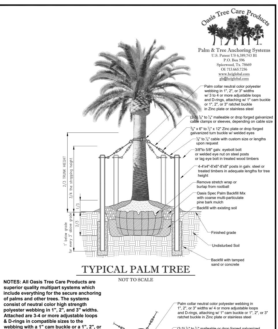
(2-3)  $\frac{1}{8}$  to  $\frac{1}{4}$  malleable or drop forged galvanized cable clamps or sleeves, depending on cable size
